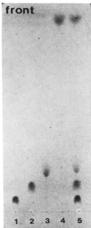
Fig. 1. Separation of 5'-ribonucleotides on Fixion 50-X8 ( H^+ ) chromatoplates in de-ionized water. Development time 60 min for 10 cm. Points show the location of samples. 1 = AMP; 2 = CMP; 3 = GMP; 4 = UMP; 5 = 1 + 2 + 3 + 4.
